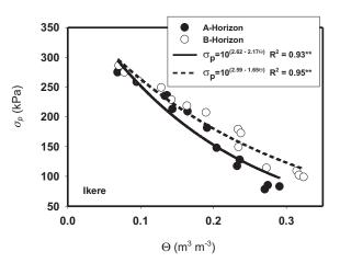
Fig. 5. Load bearing capacity curves of the studied soils.
