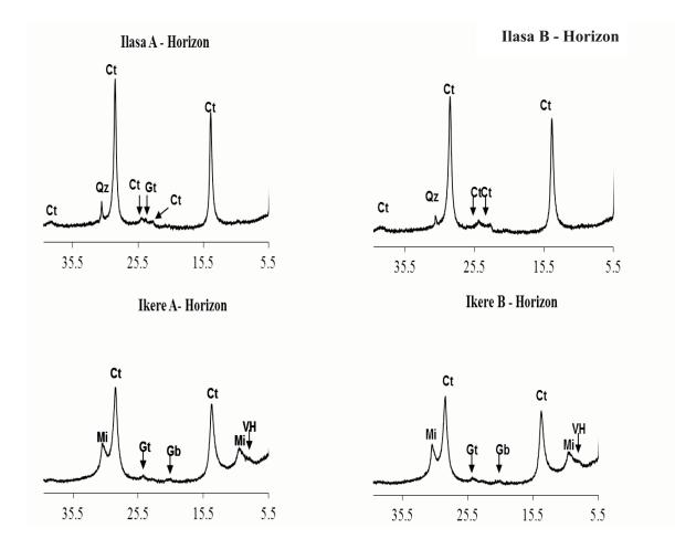
Fig. 2. Fine clay fraction X-ray diffractograms of the studied soils highlighting the mineral content and distribution. VH - hydroxy-interlayered vermiculite, Mi - mica, Ct - kaolinite, Gb - gibbsite, Gt - goethite, Qz - quartz.
